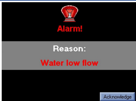
Picture 21 – Low water flow alarm
