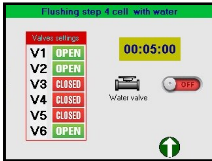
Picture 35 – STEP 4 on the PLC
